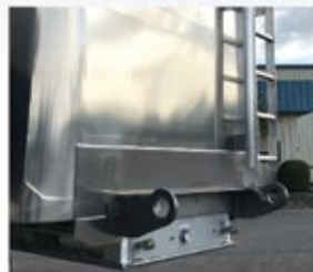
Front Ladder and Lifting Lugs for Tipping
